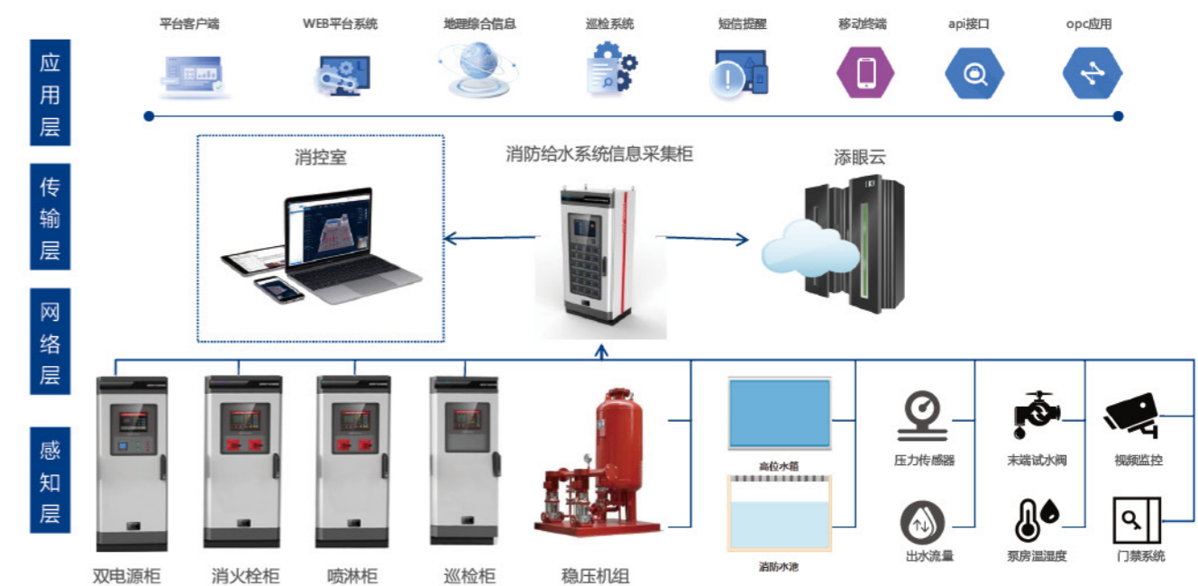
Intelligent fire water supply centralized control system architecture diagram
